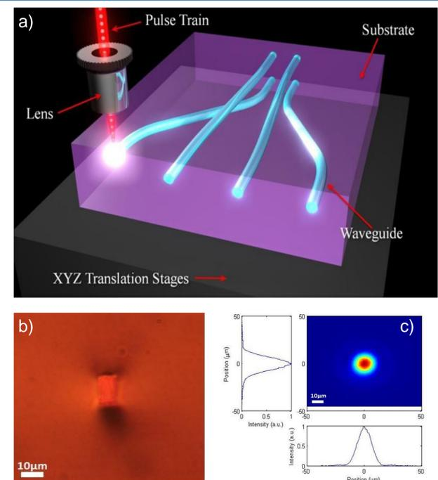
Figure 2. a) Diagram of ULI, b) Waveguide cross section inscribed in 2%Er<sup>3+</sup>:GLS via ULI, c) respective fluorescence mode at 2.73  $\mu\text{m}$
