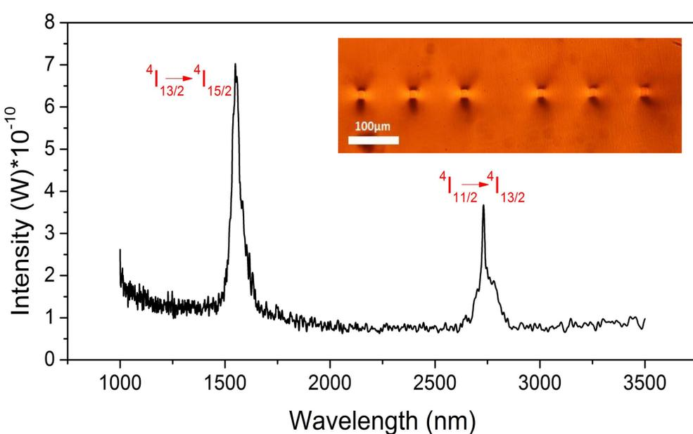
Figure 3. 1.55  $\mu\text{m}$  and 2.73  $\mu\text{m}$  fluorescence spectra for 1%Er<sup>3+</sup>:GLS and waveguide images inscribed in 1%Er<sup>3+</sup>:GLS.
