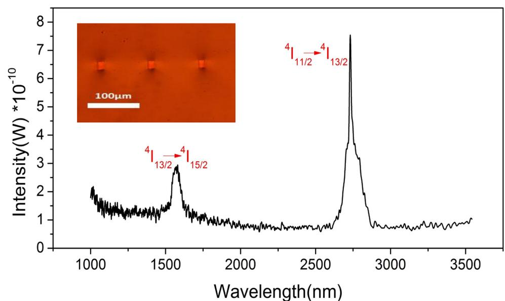
Figure 4. 1.55  $\mu\text{m}$  and 2.73  $\mu\text{m}$  fluorescence spectra for 2%Er<sup>3+</sup>:GLS and waveguide images inscribed in 2%Er<sup>3+</sup>:GLS.
