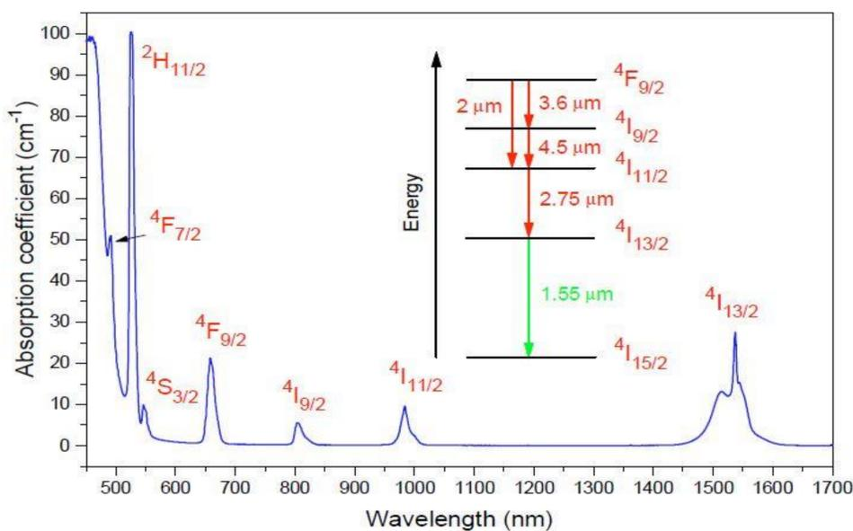
Figure 1. Absorption spectrum of 9.7mol% Er<sup>3+</sup> doped GLS glass and Er<sup>3+</sup> energy levels indicating the infrared transitions. (Reference 5)
