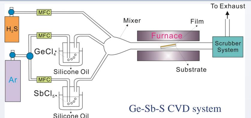
Figure 3. Schematic diagram of CVD system used for Ge-Sb-S thin film deposition.
