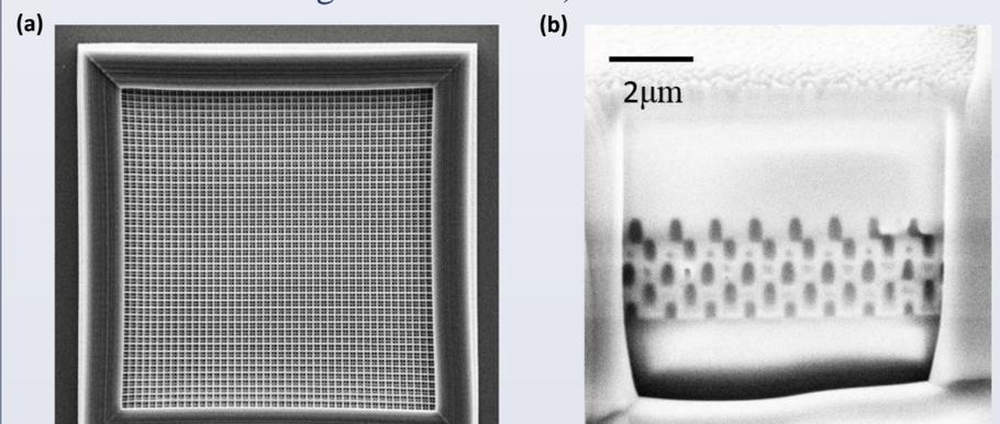
Figure 4. (a) woodpile structure template before backfill process; (b) an SEM cross-section image fabricated by focused ion beam showing the quality of infilling.
