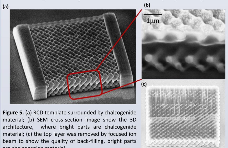
Figure 5. (a) RCD template surrounded by chalcogenide material; (b) SEM cross-section image show the 3D architecture, where bright parts are chalcogenide material; (c) the top layer was removed by focused ion beam to show the quality of back-filling, bright parts are chalcogenide material.
